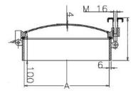
Material: Finish: \*150 - 250mm Diameter suitable for -1 to +15 bar18mm Lid Thickness8mm Thick Neckring
